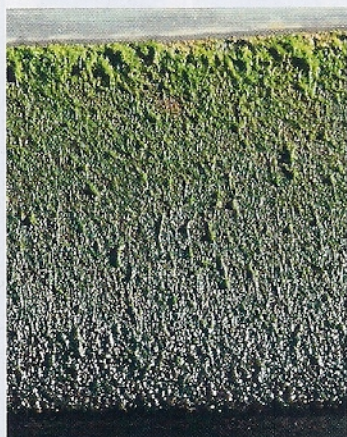
The waterline suffered a light layer of green that easily wiped away
