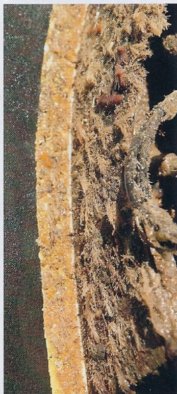
The unpainted strip on the transom was showing signs of hard fouling
