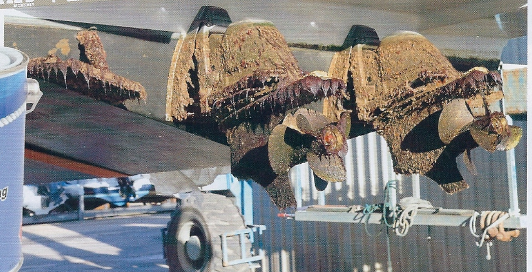
The unpainted trim tabs and stern drives provide a glimpse of just how well the hull antifoul worked
